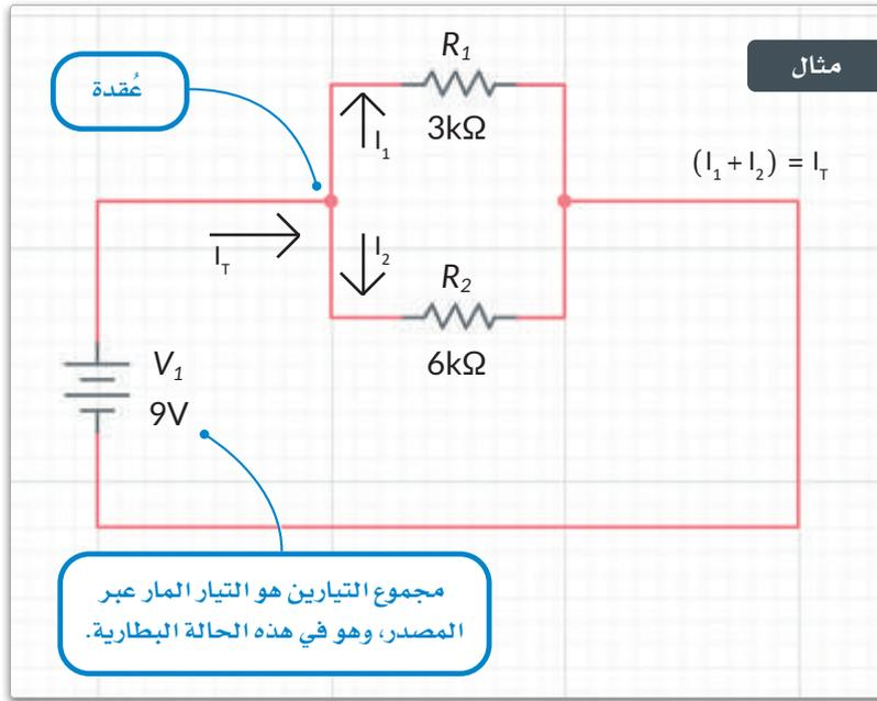
$$\frac{1}{R_T} = \frac{1}{R_1} + \frac{1}{R_2} \Rightarrow R_T = \frac{R_1 \times R_2}{(R_1 + R_2)} \Rightarrow R_T = \frac{18k\Omega}{9k\Omega} = 2k\Omega$$
