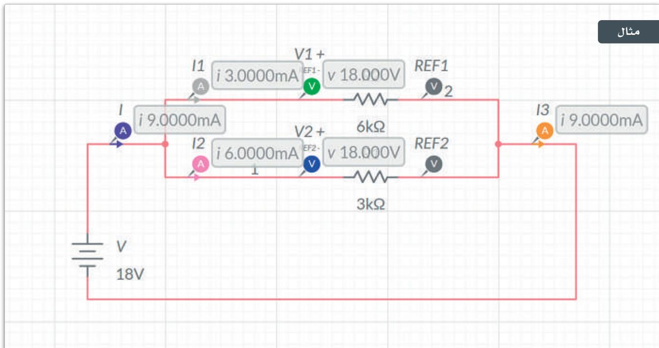
$$V_T = V_1 = V_2 = 18V$$
