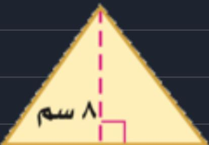
$$\begin{aligned} u &= 8 \text{ سم} \\ q &= 12 \text{ سم} \\ m &= \frac{1}{2}qu \\ m &= \frac{1}{2}(8 \times 12) = 48 \text{ سم}^2 \end{aligned}$$
